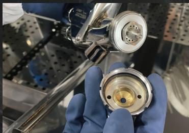
During the entire automatic cleaning process, the spray gun must not be disconnected from the compressed air coupling and must only be opened when correctly seated on the spray gun nozzle.
